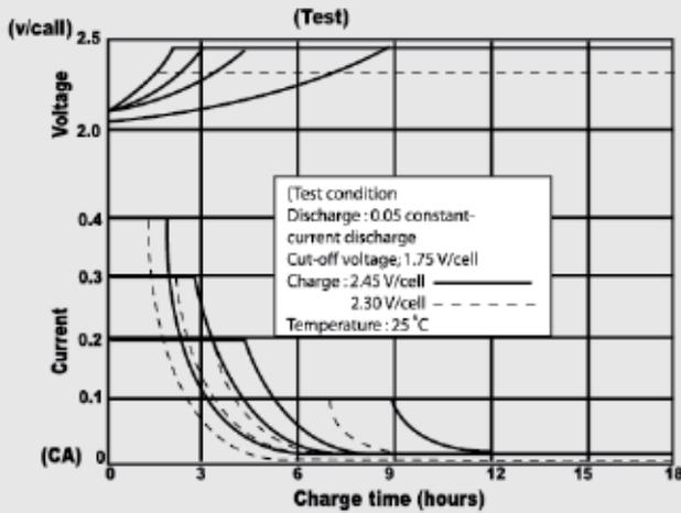
In order to fully utilize the characteristics of SLA batteries, constant-voltage charging is recommended
